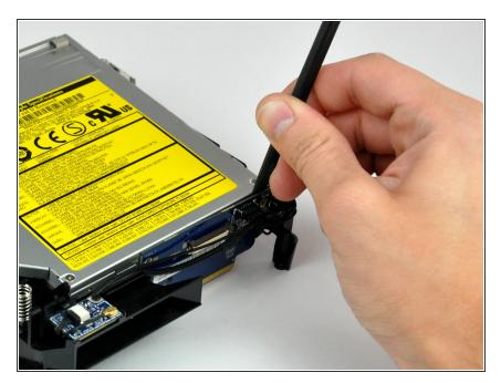
Use the flat end of a spudger to separate the interconnect board from the optical drive.
