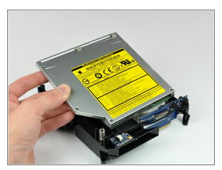
• Lift the optical drive out of the internal frame.
