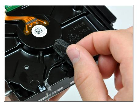
Remove the piece of foam tape covering the hard drive thermal sensor.
