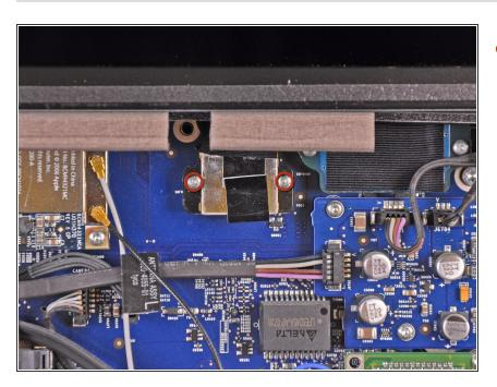
Remove the two 5.3 mm T6 Torx screws securing the display data cable to the logic board.
