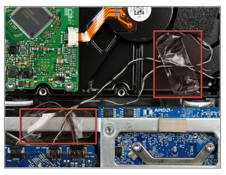
i If necessary, remove the pieces of tape securing the hard drive/optical drive thermal sensor cables to your iMac.
