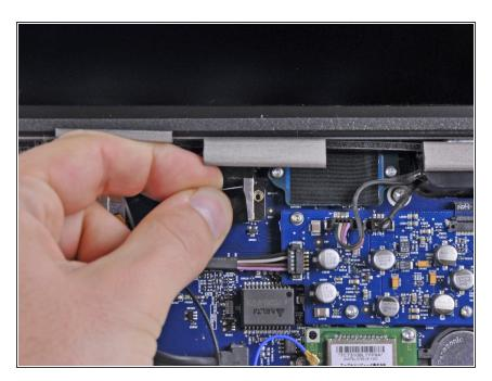
Disconnect the display data cable connector from its socket on the logic board by pulling the attached plastic tab towards you and away from the iMac.
