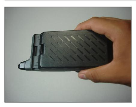
Remove the old battery by sliding it down the rails that it connects to.
