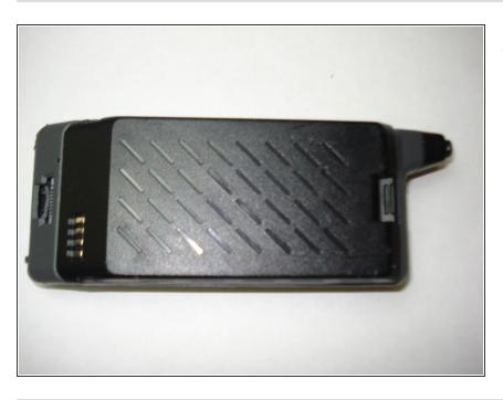
Continue sliding until the battery snaps into place. It should be secure and immobile when completely installed.
