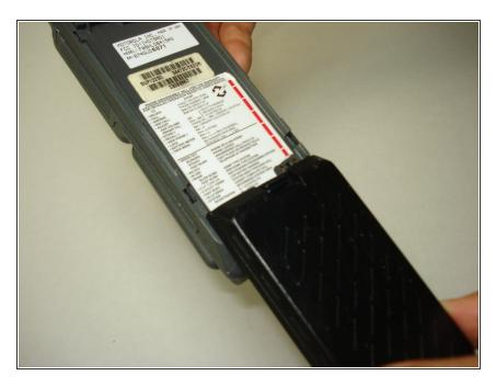
With the back of the phone exposed, align the top of the new battery with the bottom end of the phone rails.
