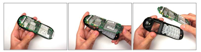
• Remove the motherboard by lifting it up and out.
