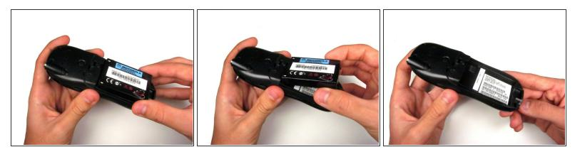
• Remove the battery by pushing the bottom end towards the top, then lifting up.
