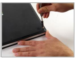
Remove the ten 10 mm Phillips #0 screws found on the computer's back case.
