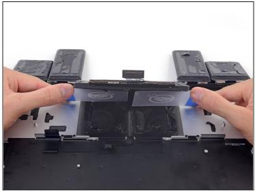
With one plastic card underneath each of the two center battery cells, twist and lift both cards to fully separate the battery cells, together with the plastic frame and battery board, from the MacBook Pro.
