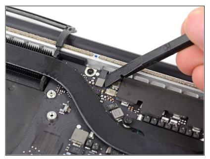
Use the flat end of a spudger to pry the keyboard backlight connector up from its socket on the logic board.
