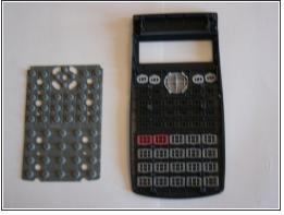
• Peel off the rubber button holder starting in the top left corner.
