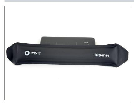
Once you have the tool firmly inserted into the glass, <u>reheat</u> and reapply the iOpener to soften the adhesive.
