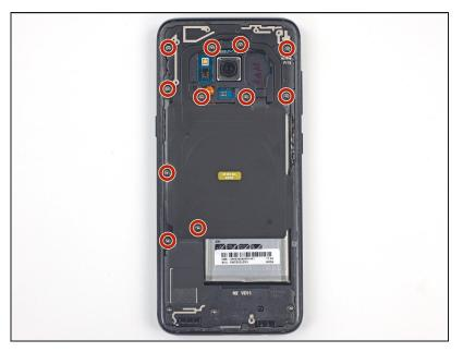
Remove eleven 3.7 mm screws using a Phillips #000 screwdriver.
