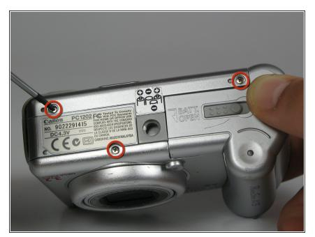
• Remove the three 2.5mm screws on the bottom of the camera.
