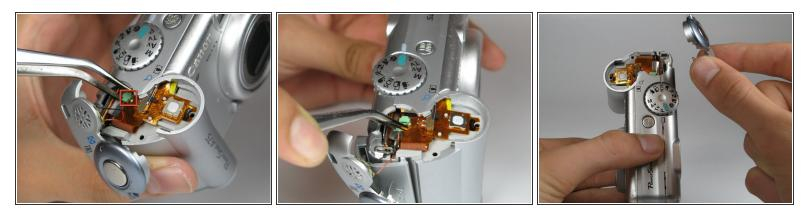
Using a pair of tweezers, grab the plug that connects the speaker to the camera and gently pull it out.
