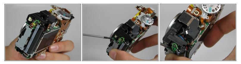
Rotate the camera such that the flash unit and capacitor are facing you.
