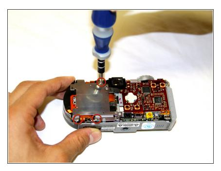
Remove the three 4.0mm Phillips #000 screws holding the back panel in place.
