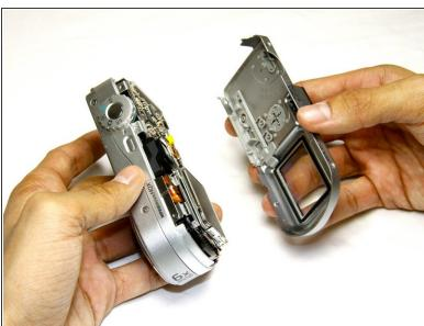
Once the screws are removed, slowly remove the back casing from the rest of the camera.
