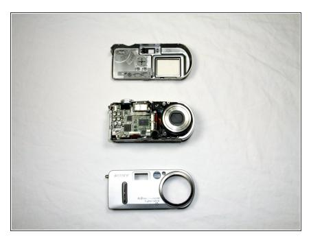
After the casing is removed, the camera should look as shown.
