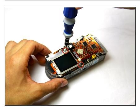
Unscrew the two 4.0mm Phillips #000 screws from the display.
