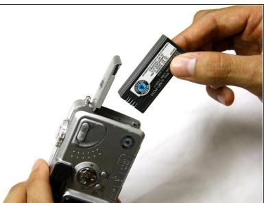
Remove the battery from the camera.
