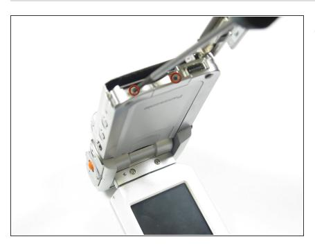
Remove the two screws (2.2mm Philips) indicated.
