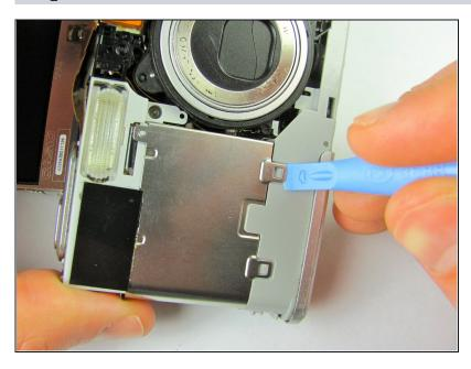
Using the plastic opening tool, pry the battery case clamps (located on front of the camera) so that the bottom portion of the camera will come loose.
