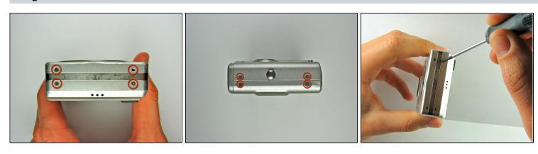
Remove eight 1.8 mm screws from the left and right sides of the camera using a Phillips #00 screwdriver
