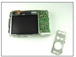
Remove the metal grating located to the right of the LCD screen by inserting the plastic opening tool under the grating and pulling up.
