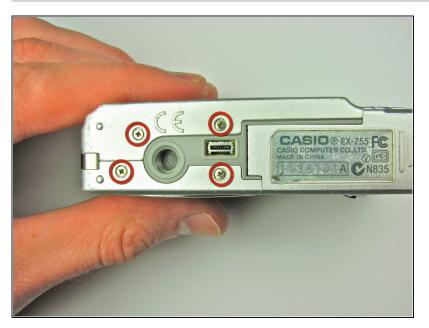
Remove the four 3.7 mm screws from the bottom of the camera using a Phillips #00 screwdriver.
