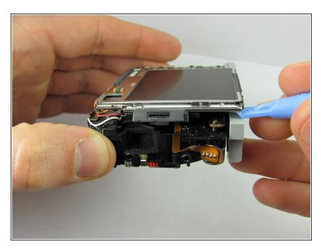
Using the plastic opening tool, pry up the LCD screen starting at one of the corners. Insert the tool under one of the corners and lift up.
