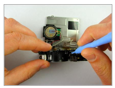
Detach the inner orange ribbon cable that connects the motherboard to the lens by inserting the iFixit plastic opening tool under the tab and lifting up.
