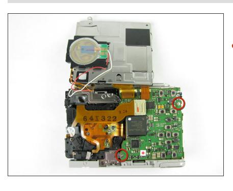
Remove the two 1.7 mm screws from the motherboard using a Phillips #00 screwdriver.
