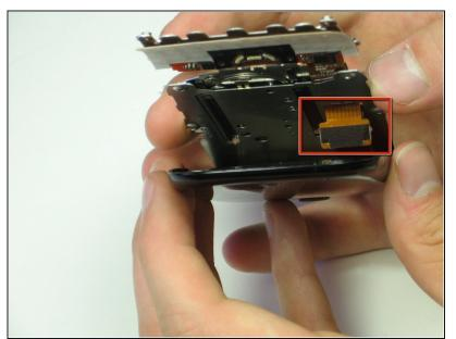
• Remove the two ribbon cable connectors using <u>tweezers</u>.
