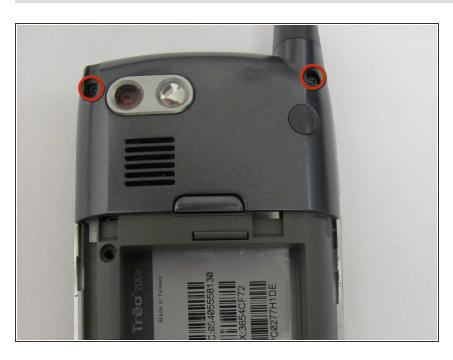
• Unscrew the last two screws using the same T-5 Torx screw driver.
