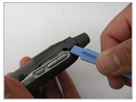
Using the plastic opening tool, carefully pry open the back case to loosen the antenna.
