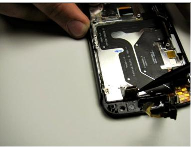
Using a spudger, lift up the digitizer cable that is attached to the glass.
