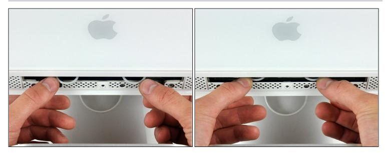
(*i*) Orient the iMac face-up, on its backside.
