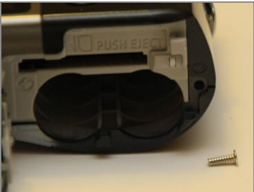
• The last coarse thread screw is located under the battery/memory card cover. Remove this screw and we will be ready to open this baby up!
