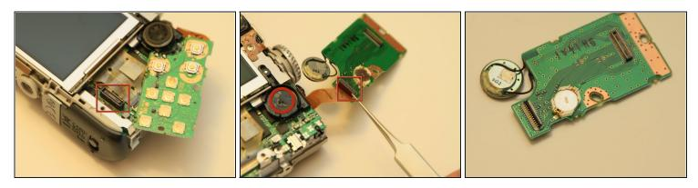
• Gently lift the keypad up from the bottom to remove it from the connector shown. You may need to pry up the speaker from it's holder, it is held in place with double-sided tape. Lift the keypad upside down and unhook the connector by lifting the gray cam and removing the flexible cable.
