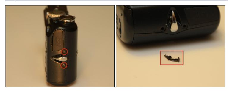
• On the left side, remove the two coarse thread screws.
