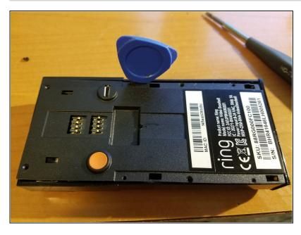
Carefully pry the plastic coverwith a pick to pop the insert out. Watch the micro USB port that is sticking out.
