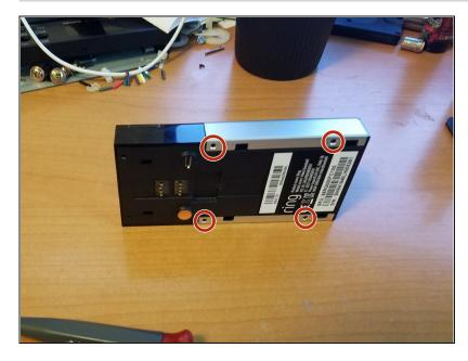
Start by removing the 4 screws to take off the aluminum faceplate.
