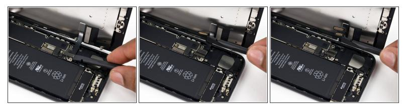
Make sure the battery is disconnected before you disconnect or reconnect the cables in this step.
