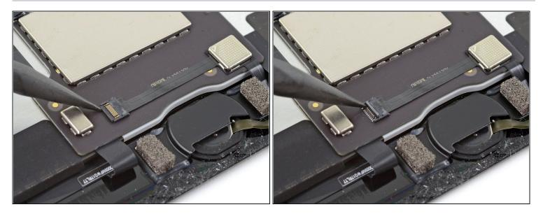
• Use the point of a spudger to lift the flap on the ZIF connector that secures the cable.
