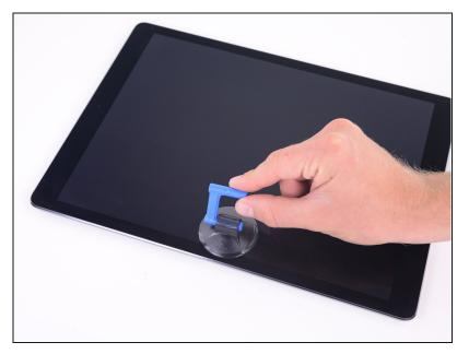
Attach a suction cup to the left edge of the iPad's screen, above the Smart Connector port.
