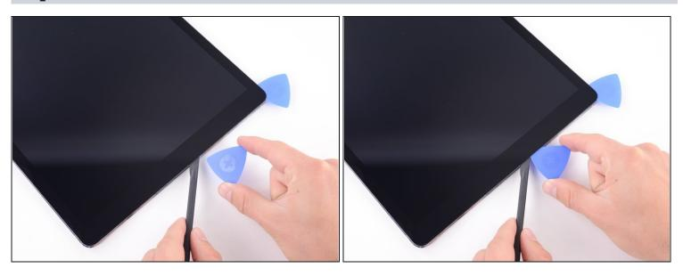
Insert an opening pick just before the front-facing camera to keep the adhesive from resealing.
