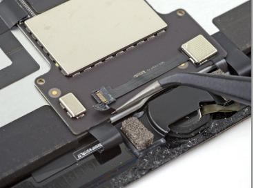
• Use tweezers to remove the tape covering the ZIF connector above the home button.
