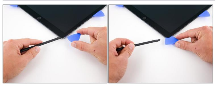
• Leave an opening pick in the lower right corner of the iPad to prevent the adhesive from resealing.
