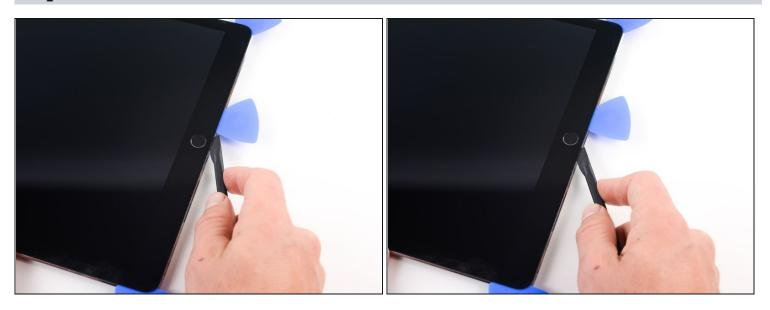
• Slide the tip of an opening pick or a halberd spudger to cut the adhesive below the home button.
