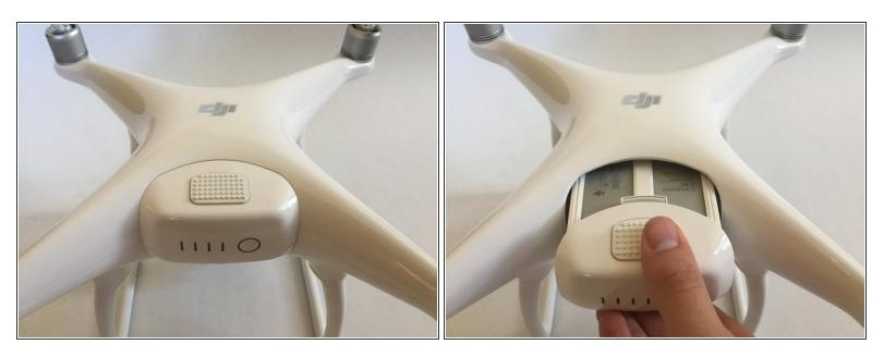
• Firmly press the battery tabs on top and bottom of the battery and slide out the battery.
