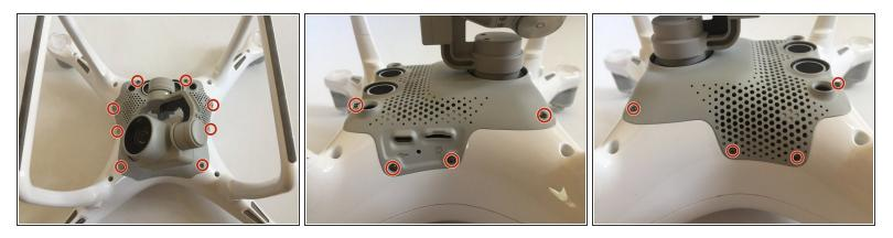
Using a T6 screwdriver, remove all eight screws on the grey gimbal assembly.
