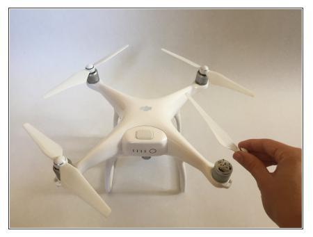
Push down and twist the propellers counter-clockwise to release from the drone.
