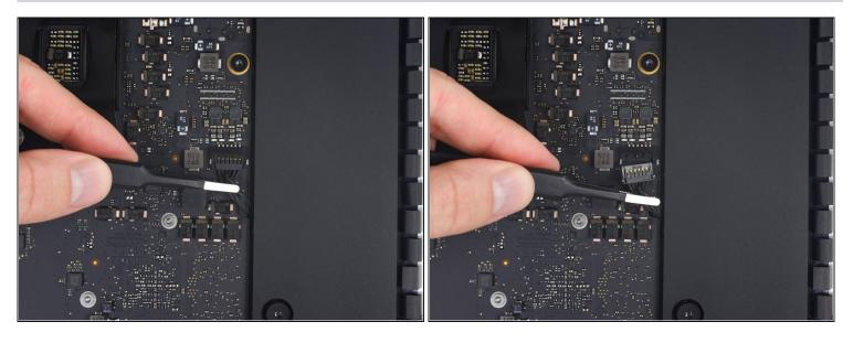
• Gently pull the right speaker cable connector straight down and out of its socket on the logic board.
