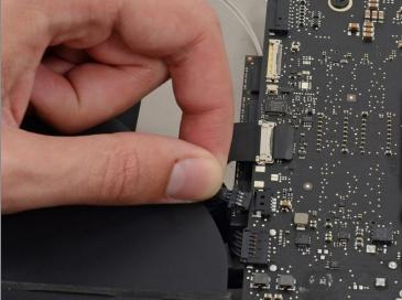
• Gently pull the fan cable connector straight out of its socket on the logic board.
