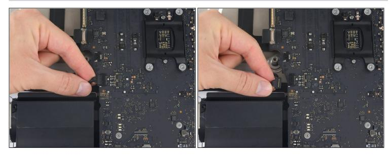
• Gently pull the left speaker cable straight out of its socket on the logic board.
