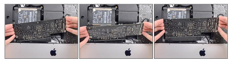
• Rock the power supply forward and remove it from its recess in the rear enclosure.
