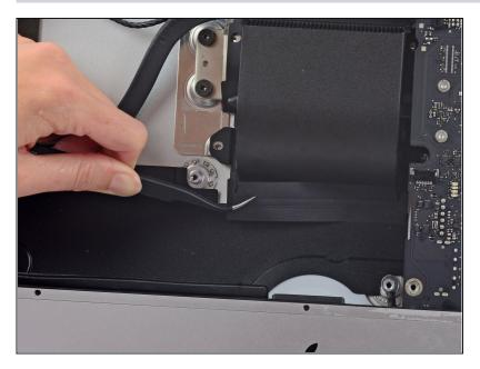
Peel off the tape covering the exhaust duct.
