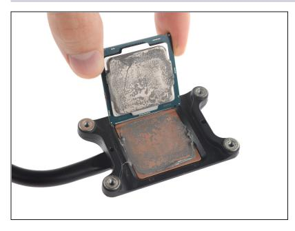
• Lift and remove the CPU from the heat sink.
