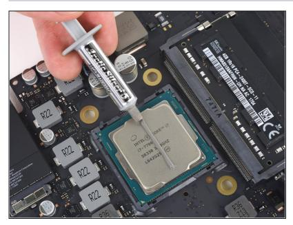
• Follow the instructions specific to your CPU type to apply fresh thermal paste to the surface of your CPU.
