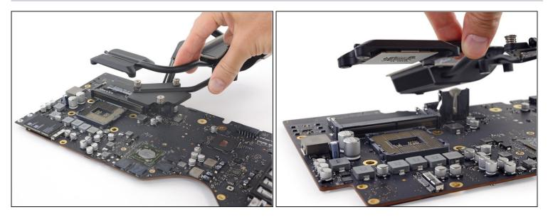
⚠️ Note that the CPU will most likely remain stuck to the underside of the heat sink as it's lifted out. Take care not to damage it.
