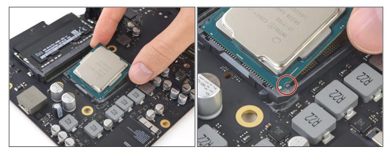
Check the orientation of your CPU before installing it.
