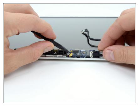
Use the tip of a spudger to disconnect the two antenna cable connectors from the AirPort board.
