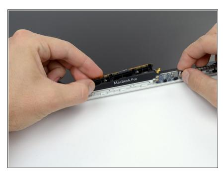
• Lift and remove the AirPort antenna from the display case.
