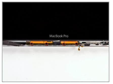
Remove the four 4.0 mm Phillips #00 screws securing the AirPort antenna to the display case.
