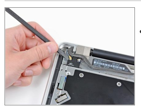
Use the flat end of a spudger to pry the Bluetooth antenna connector up and off its socket on the Bluetooth board.
