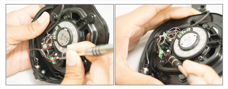
Remove the two 2 mm long screws securing the motherboard using a Phillips #000 screwdriver.
