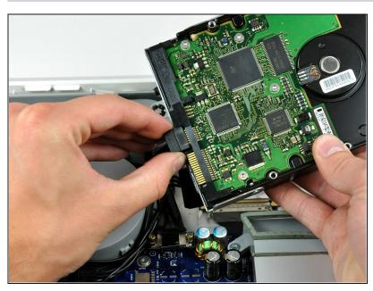
Pull the SATA data cable connector away from the hard drive.
