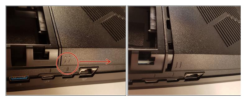
• Slide the plate in the direction of the red arrow.
