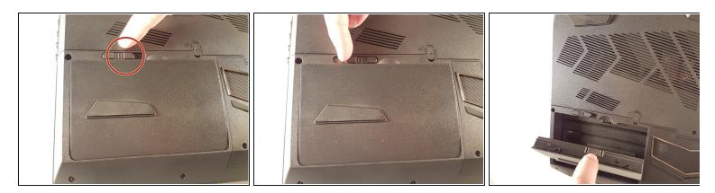
• Lift the battery while unlocking the lock circled in red.
