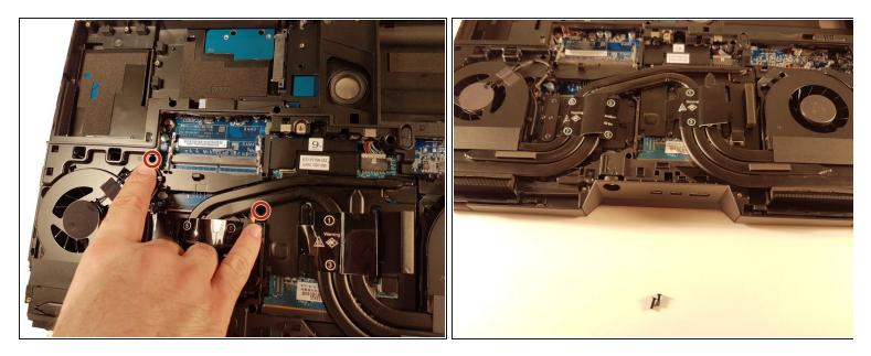
• Unscrew the two screws circled in red
