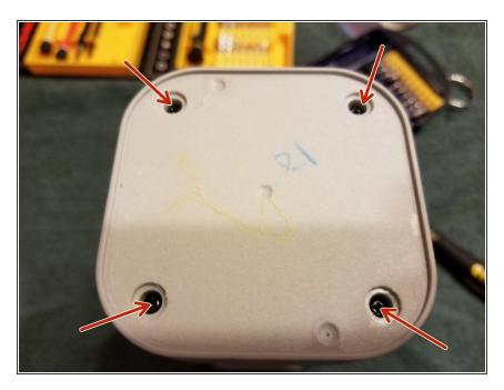
User #1 Phillips screwdriver to remove 4 screws from the bottom.
