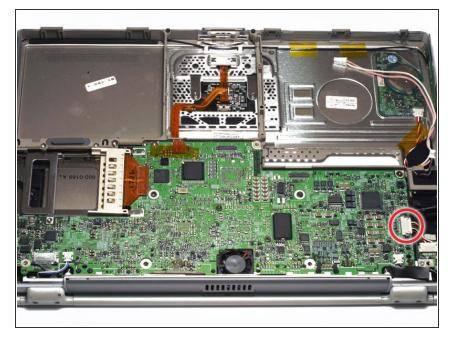
Disconnect the large DC-In connector from the right side of the logic board.
