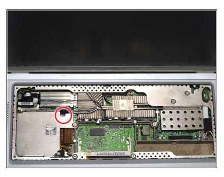
Remove the T8 Torx screw near the heat pipe.
