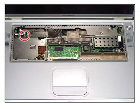
Remove the T6 Torx screw from the modem filter board.
