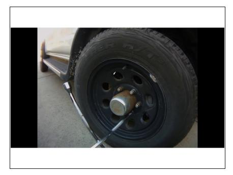
• <u>Loosen all six</u> lug nuts on the passenger side wheel before jacking up the vehicle .
