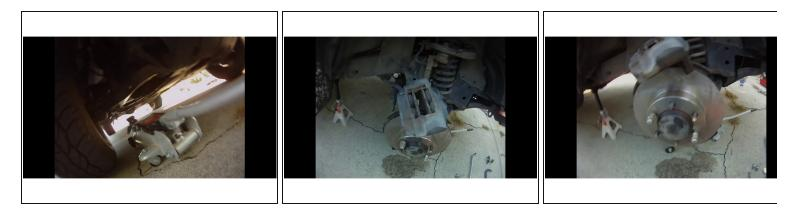
• <u>Remove the pins</u> holding the old brake pads in place and take out the old pads .
