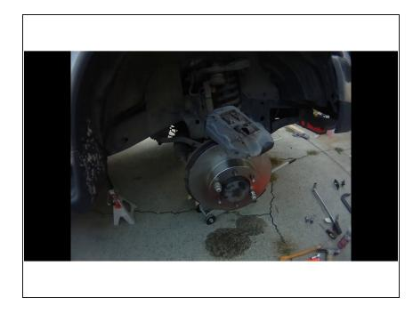
• <u>Install the new</u> rotor and secure it in place using two lug nuts to align it correctly .
