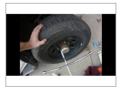
• <u>Tighten the lug</u> nuts before lowering the vehicle back onto the ground .
