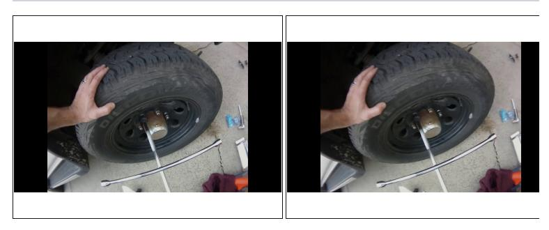
• <u>Remove the two</u> lug nuts used to align the rotor and put the wheel back on .
