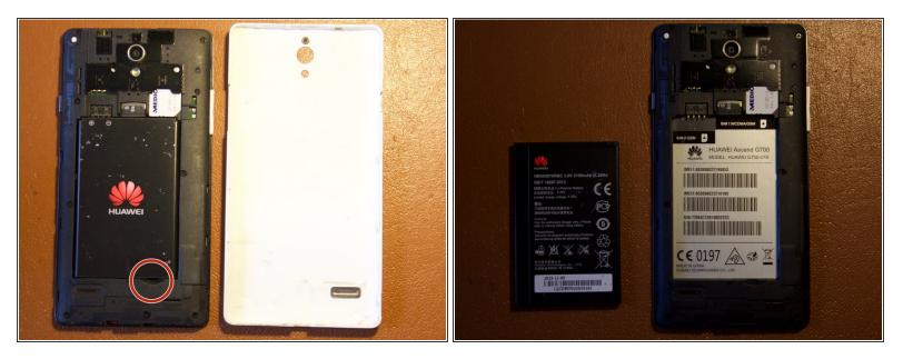
• Now you can remove the battery, that has to be pryed off in the marked location.
