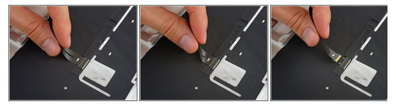
• Gently peel the keyboard ribbon cable up from the case, and remove the cable.
