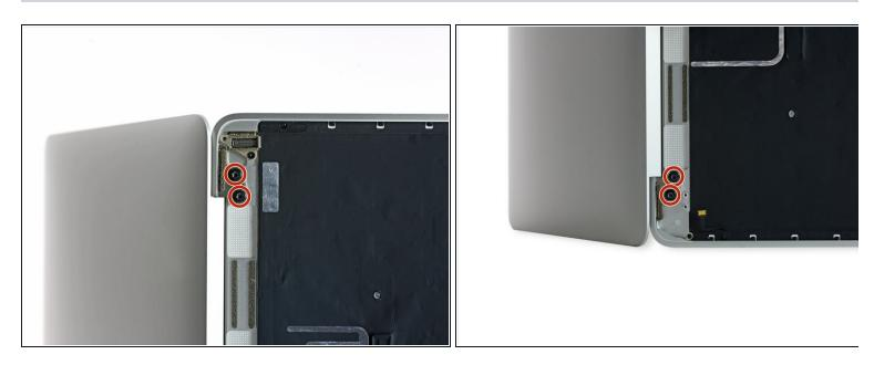
• Remove the four 4.8 mm T8 Torx screws securing the display hinges.
