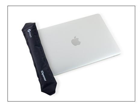
Prepare an iOpener and apply heat to the upper case directly behind the microphone assembly.
