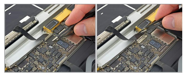
• Use tweezers to peel back the tape covering the display cable connector.
