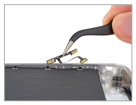
• Remove the dual microphone assembly.
