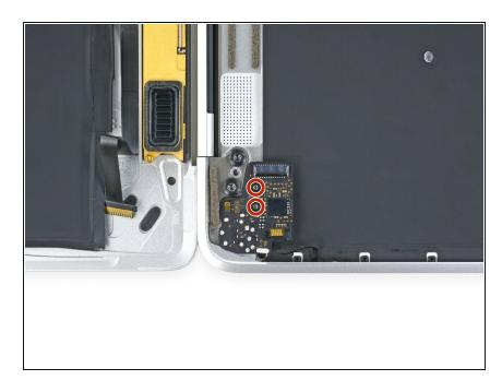
Remove the two 3.2 mm T5 Torx screws securing the audio jack board to the case.
