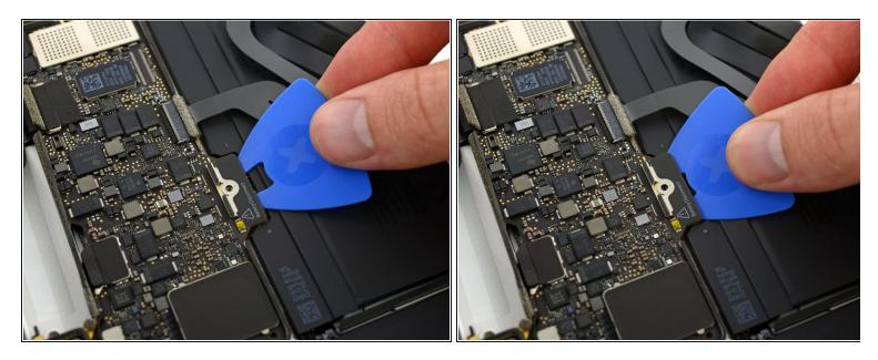
As an added precaution, you may physically disconnect the battery by inserting a <u>battery</u> <u>isolation pick</u> between the logic board and the battery connector.
