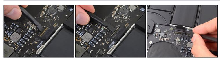
• Use the flat end of a spudger to flip up the retaining flap on the keyboard ribbon cable ZIF socket.
