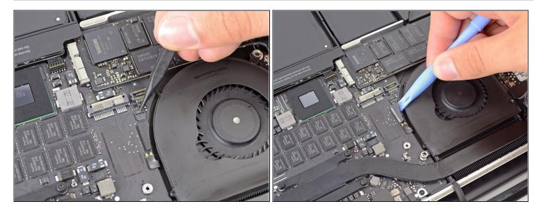
• Use the tip of a spudger to flip up the retaining flap on the right fan ribbon cable <u>ZIF</u> socket.
