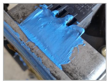
Use silicone to reattach the cover plate and to seal up the side access hole. Allow the silicone to set up before reinstalling the throttle body to the engine.
