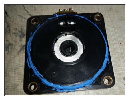
Reassemble the metal ring. Apply silicone adhesive around the outside edge, then reinstall the sensor into the throttle body.
