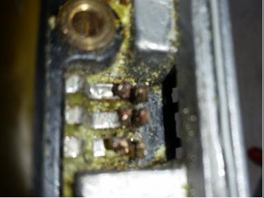
Dig the silicone sealer out of the right side to expose the position sensor wire terminals. The terminals are spot welded (yes, WELDED) together to the leads from the computer module. Use small sharp diagonal cutters to separate the terminal leads.
