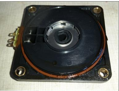
The inside of the housing and the position sensor will both have an oily mess. Clean them by spraying with carb spray or contact cleaner.
