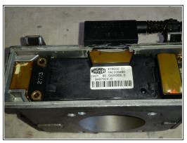
• Remove the throttle body from the engine. Remove the cover plate by prying up on the edges with a small screwdriver. It is glued down with silicone. Under the cover plate you will see a computer module that is also siliconed in place.
