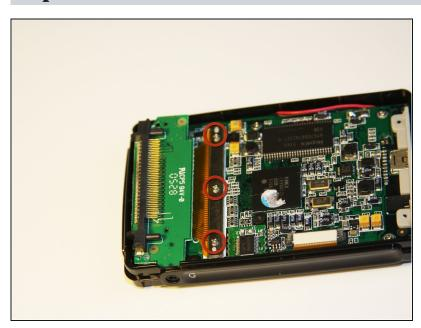
Using the Phillips #00 screwdriver, unscrew the three 1.5mm long screws on the metal bracket.
