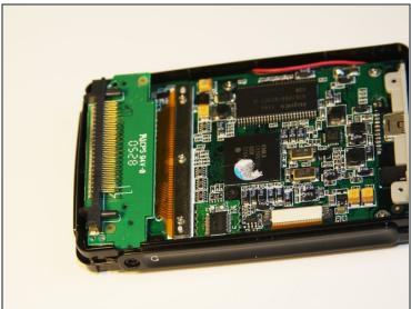
• Using the Phillips #00 screwdriver, unscrew the two 1.5mm long screws holding the IDE connector to the motherboard located at the top.
