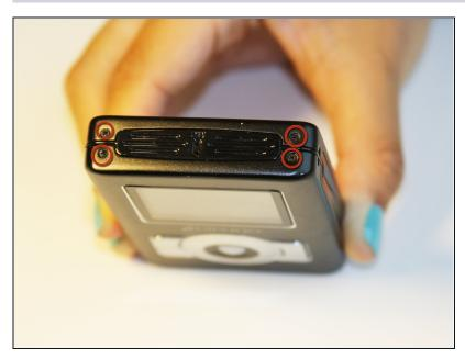
Use a Phillips #00 screwdriver to unscrew the four 1.1mm long screws on each corner located at the top of the cover.
