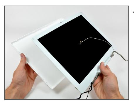
Lift the rear bezel off the display.
