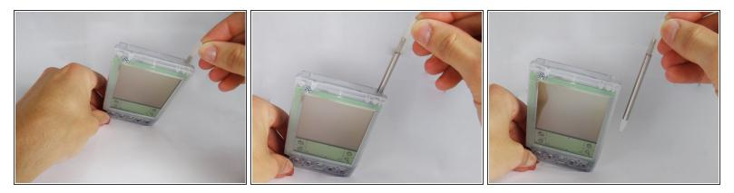
• Pull out the stylus from the top right corner of the device.
