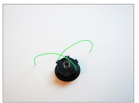
If there are plastic tabs on the plastic part to hold the cutting line, insert each line into one these tabs. Leave approximately a foot of each line hanging out from the coils.
