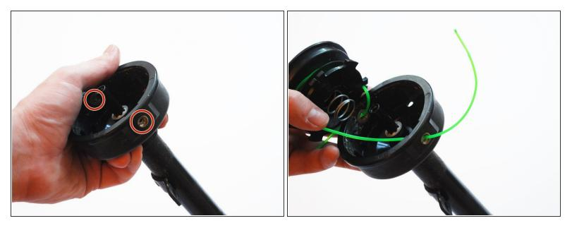
On the weed whacker rotor, there will be eyelets for the cutting line to be fed through. Feed each line through each of these eyelets, being careful not to let the line come uncoiled.
