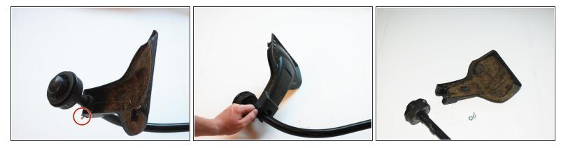
• Remove cutting line guard from weed whacker. This is usually attached by a wing-nut or a bolt and nut, so it can be removed either by hand or with the correct sized wrench.
