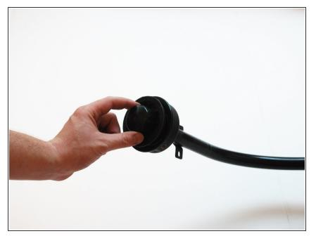
There will be a bottom cap of the rotor setup that needs to be removed. In some models this will be held on with a nut and bolt fixture, but in many models there will be a circular cap that can be rotated counter clockwise for removal. Remove this piece in the manner necessary.
