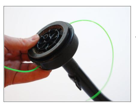
Replace the plastic piece with the cutting lines back onto the rotor, being sure that the coils remain in place, and the lines remain in place through the eyelets.
