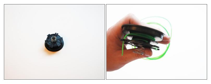
• There should be slots to coil cutting line around, with a hole in each for line to be anchored. If no line is coiled around the part, insert the end of about three feet of cutting line into each of the holes, and coil the cutting line snugly around the part, making sure that there are no tangles in the line.
