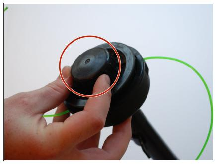
• Replace the cap that was removed at the beginning of the assembly.
