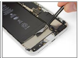
Peel back the first battery adhesive tab from the bottom right edge of the battery.
