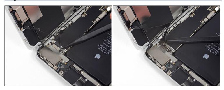
• Use the tip of a spudger or a fingernail to disconnect the front panel sensor assembly connector from its socket.
