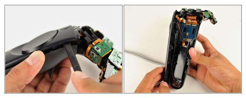
Use the nylon spudger to separate the front panel gently by running the spudger around the edges of the handle.
