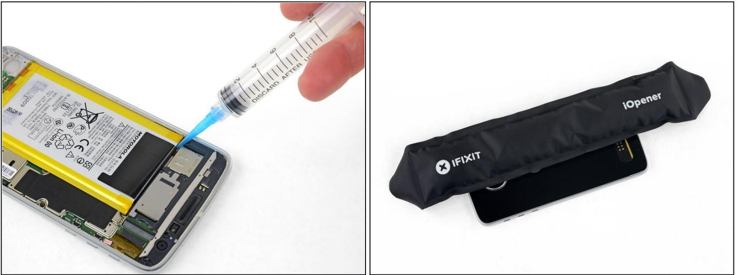
ⓘ The battery is strongly glued into place.
