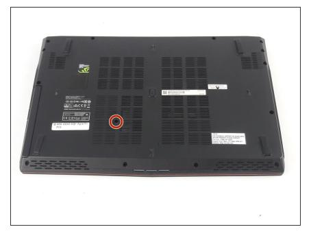
Use a Phillips screwdriver to remove the 5mm screw securing the optical drive to the bottom case.
