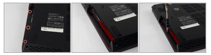
• Remove the three PH #0 2mm screws that were hidden underneath the optical drive.
