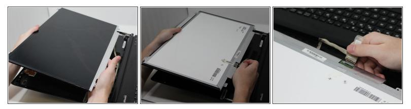
• Flip the screen over and carefully peel off the tape that holds the connector in place.
