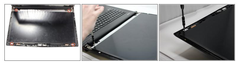
• Using the Phillips #0 screwdriver, remove the four 3mm long screws.
