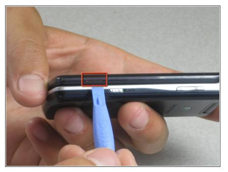
Find the small notch on the side of the phone. The notch is located by the "fast-forward" button and the "lock" switch.
