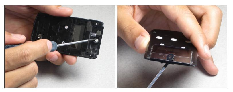
• Remove the lends by pushing the lens from the inside of the housing.
