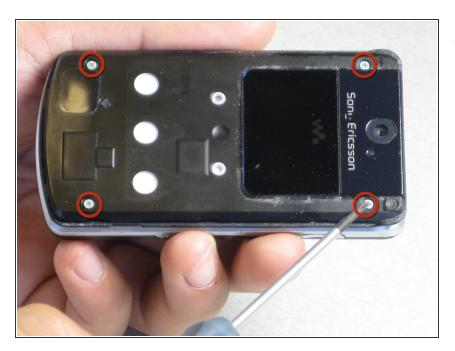
Remove the four 2mm Phillips screws from the back housing of the phone.
