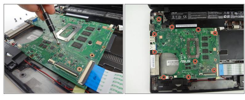
Remove the 10 black 4.7mm screws holding the motherboard/RAM in place using a Phillips #00 screwdriver.
