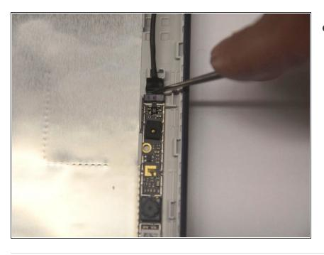
Using the spudger, disconnect the cable from the camera. The camera will then pop out.
