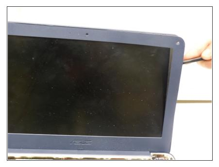
Using the plastic opening tool, carefully pry off the bezel. It will come off entirely, so be careful not to break it.
