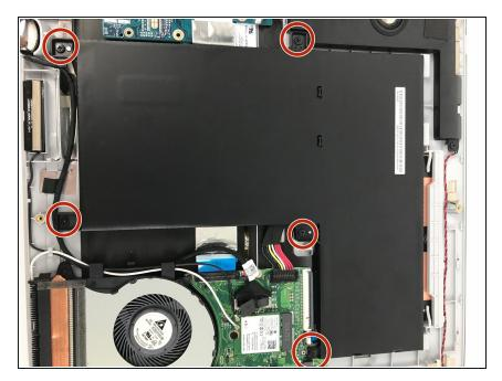
Use the Phillips #0 screwdriver to remove the five 4mm screws around the battery.
