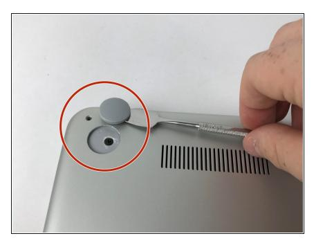
Remove the two rubber pads nearest to you using the metal spudger.
