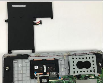
Remove the battery from the device.
