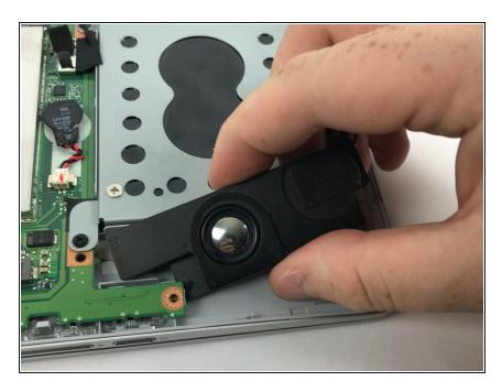
Remove the Right (R) speaker from the device. Using a spudger helps to slide it out.
