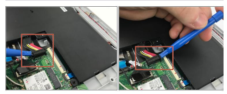
• Use the small plastic opening tool to remove the ZIF Connector on the right side of the battery.
