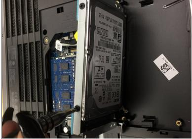
Unscrew the four screws on the long sides of the hard drive casing
