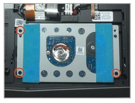
Remove the screws that connect the SSD Bay to the laptop
