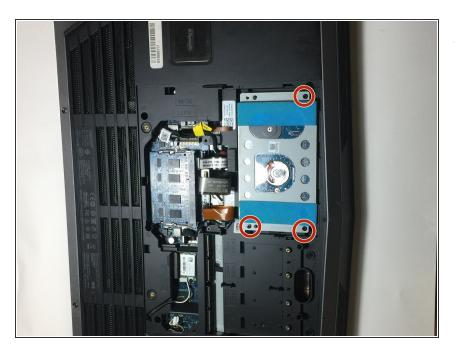
Unscrew the three screws holding the hard drive
