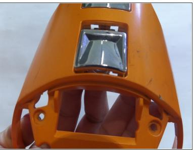
When placing new button in make sure the bottom end goes in first.
